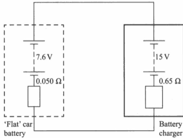
The positive terminal of the car battery is connected to the positive terminal of the battery charger.
