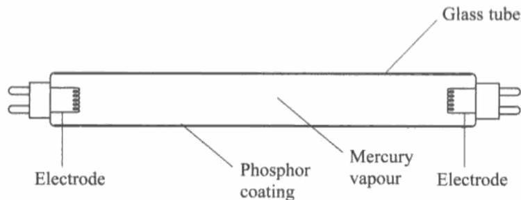
When the light is switched on, charge flows between the electrodes and the mercury atoms become excited. The mercury atoms then emit electromagnetic radiation.
